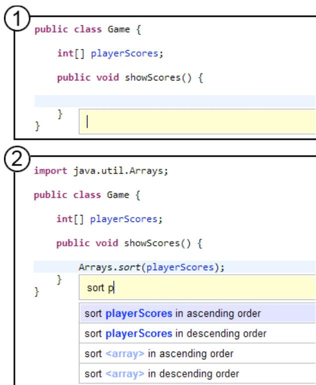
**Figure 1.** The SnipMatch plug-in for the Eclipse development environment. A keyboard shortcut opens the search window (1) at the programmer's cursor position. Search results (2) are updated as the query is typed. The search query also affects integration: the local variable `playerScores` is included in the snippet (2). Snippet integration is previewed within the existing code.
